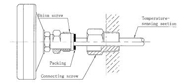
(2) Installation of the thermometer must be made without fail by fastening the hexagonal part with wrench but not by holding the indication section. Insert the temperaturesensing section fully into the object fluid (liquid, oil or air). Otherwise, accurate indication is impossible.
