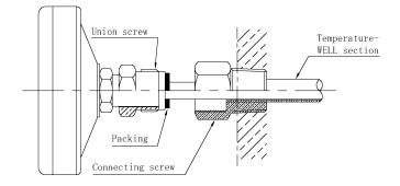
(2) Installation of the thermometer must be made without fail by fastening the hexagonal part with wrench but not by holding the indication section. Insert the temperaturesensing section fully into the object fluid (liquid, oil or air). Otherwise, accurate indication is impossible.
